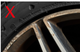
Excessive Damage to wheels
