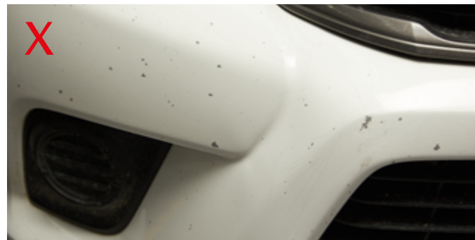
Excessive stone chipping
