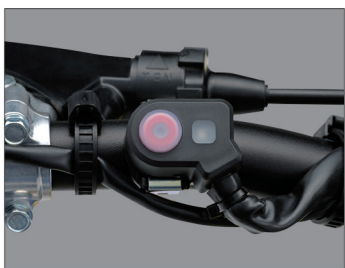
Suzuki Holeshoot Assist Control (S-HAC)
