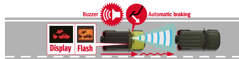
3. Applies strong automatic braking if the risk of collision increases even more.
