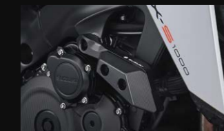
Frame slider Helps reduction of damage, made of aluminium and POM (polyacetal)
