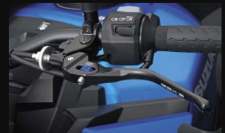
Billet brake lever (Anodized) Machined from high-end billet aluminum and decorated with the GSX-S logo, these black anodized levers enhance the bike's sporty good looks.
