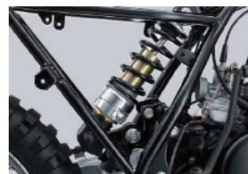
Rear suspension with mono-shock absorber
